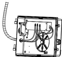
**9** The top terminal connect the wire tube through the side hole to the L,N and G wires on the power supply.
