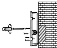
**8** Lock the bottom shell on the mounting seat with screws.
