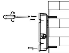
**8** Push the expansion rubber plug into the mounting hole on the wall
