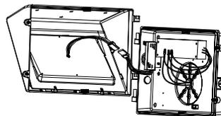
**10** Install the upper cover of the fixture and connect the terminal line.
