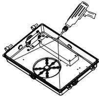
**4** Drill through the mounting hole with an electric drill.
