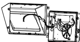
**10** Install the cover of the fixture and connect the terminal block.
