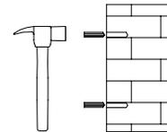
**6** Push the expansion rubber plug into the mounting hole on the wall.
