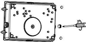
**7** Use a screwdriver to remove the side plug and attach the EVA cotton pad to the mounting hole.
