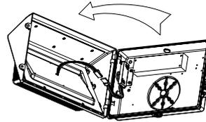
**3** Open the fixture, disconnect the connection terminals, and remove the upper cover of the fixture.
